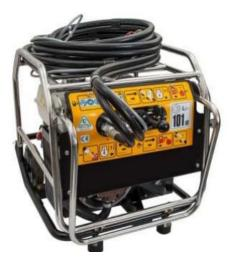
A trolley-mounted hydraulic power pack with pre-set internal system protection relief valve and quick release connectors. The unit is powered by an air-cooled, 8hp Honda GX240 petrol engine, delivering 15 litres/min at a working pressure of 115 bar from the hydraulic circuit. The circuit is protected with a return line and suction filters. The unit is mounted on a robust, wheeled trolley.
